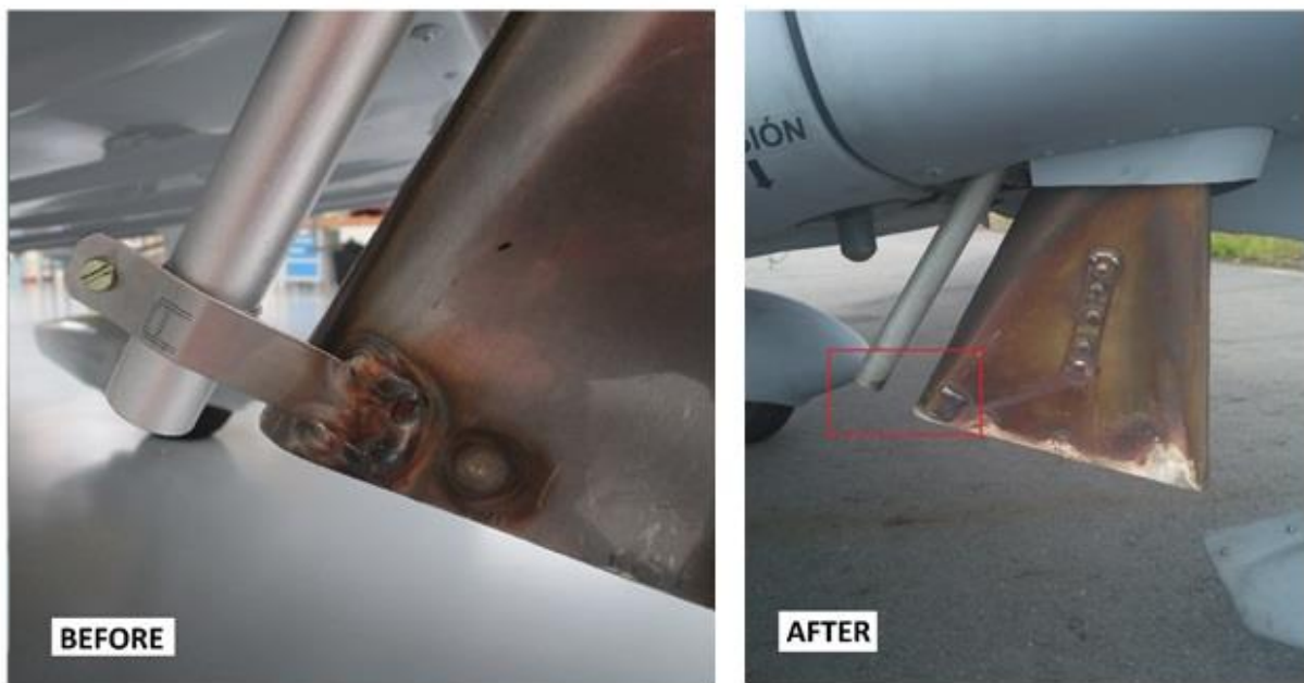
Fig. 1.1 Problem of the broken original Console L242.6674-00.17C
